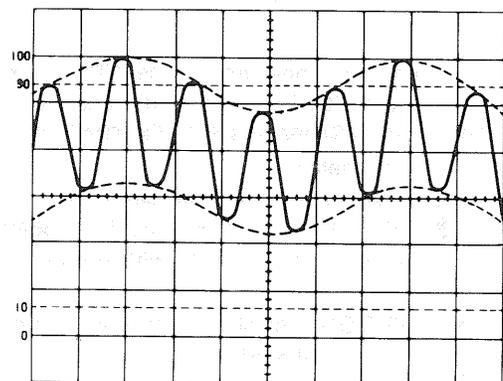
Signal containing undesired component
